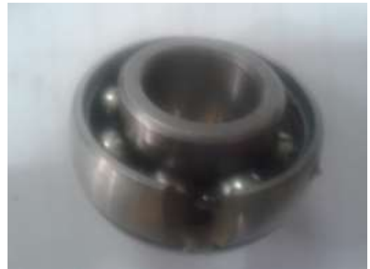
Figure2(b) Faulty Bearing
